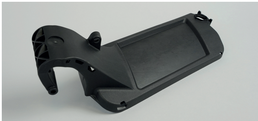
Fig. 1. Hinge arm for the tank cap of Audi vehicles: by switching to a PP with recycled carbon fibers, the weight could be reduced by 32% and the CO 2 emissions by almost 75% © Albis
